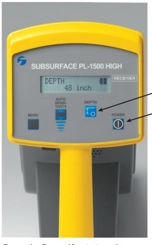
Press the Power Key to turn the receiver ON or OFF. Press the Depth Switch to measure the depth of the pipe or cable.
