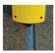
To measure the depth of the pipe or cable, first stand the receiver straight up with the black rubber tip touching the ground directly over the line. The receiver must face in the line's direction.
