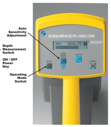
Press the Mode Switch to select the MAX Mode or the Live Cable / 60 Hz Mode. Press the Auto Sensitivity Switch whenever the sensitivity needs to be increased or decreased.
