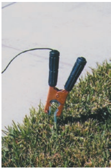
Place the Ground Stake 5 to 15 feet from the side of the conductor
