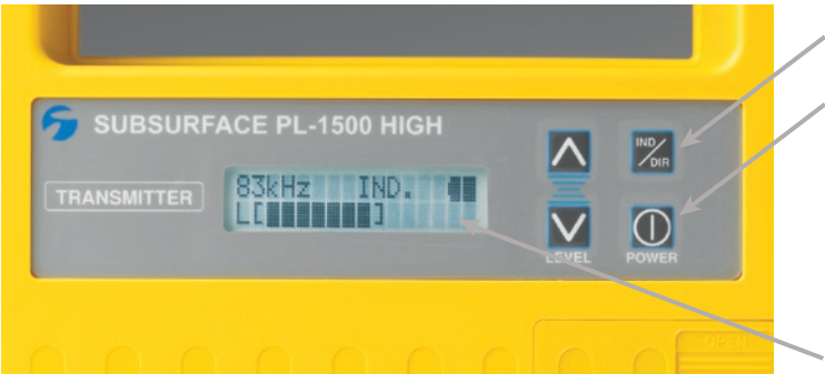
Inductive Mode / Direct Mode Switch
