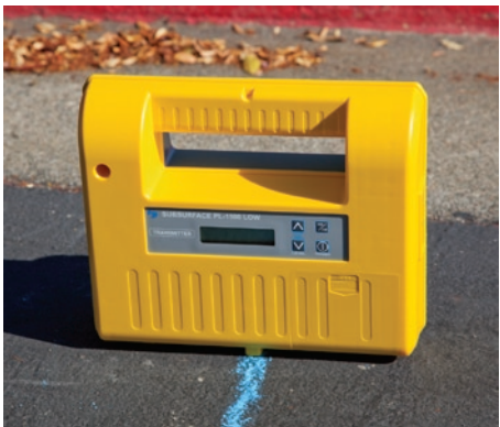
Right Way: Facing in direction of pipe or cable
