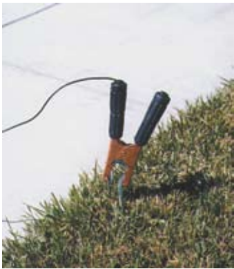
Connect Black cable to the Ground stake
