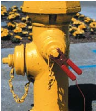
Connect Red cable to conductor
