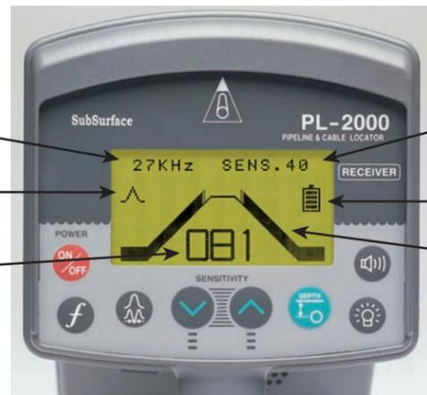
3. Select the same frequency as selected at the transmitter for "active" locating, or select "Radio" or "50/60 Hz" for "passive" locating (no transmitter).
