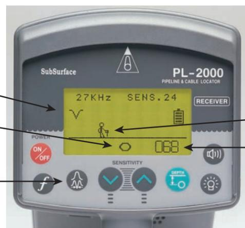
5. The receiver only locates the line in Peak Mode and DIST Mode when the bar graph is climbing on the sloped sections.
