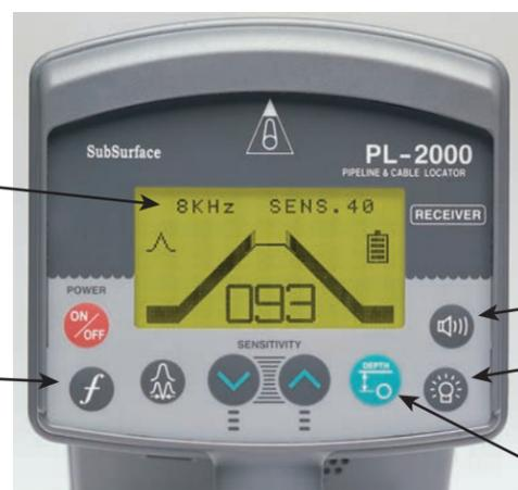
4. Select the Operating Mode depending whether you wish to locate a line with highest accuracy or longest distance, or you are locating a Sonde inside a pipe.
