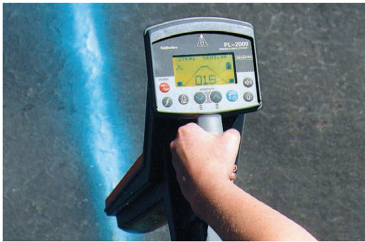
1. The Receiver must be operated facing in the direction of the pipeline or cable.
