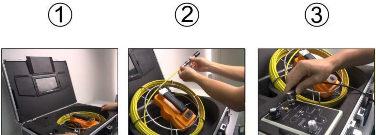
4. Connect the other end of connection wire to the cable wheel
