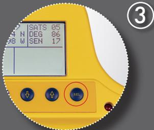
The AML Pro has a GPS tracking system that is active as soon as you turn ON your unit. It is only able to acquire public GPS satellites when you are using the All Materials Locator outdoors.
