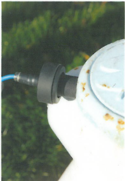
Listening at a hydrant with the magnet base
